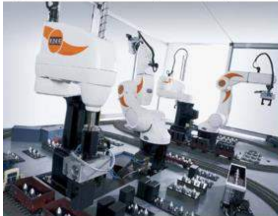
Figure 5. SCARA - Selective Compliance Assembly Robot Arm.
