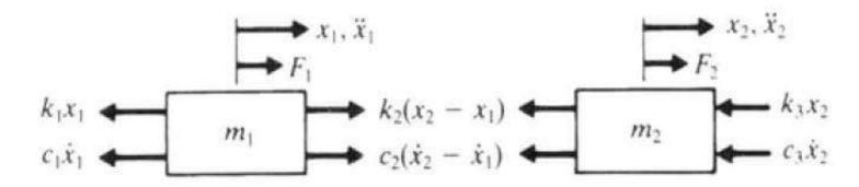
$$m_1\ddot{x}_1 + c_1\dot{x}_1 + k_1x_1 - c_2(\dot{x}_2 - \dot{x}_1) - k_2(x_2 - x_1) = F_1$$
