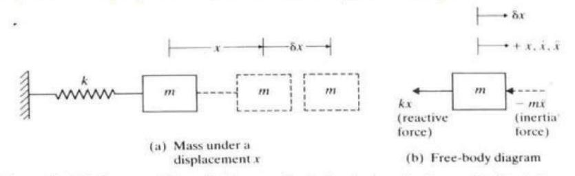
When a virtual displacement dx is applied, the sum of work done by the spring force and the inertia force are set to zero:
