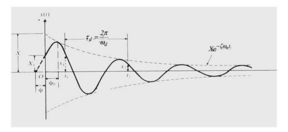
Exponentially decaying harmonic – free SDoF vibration with viscous damping . Underdamped oscillatory motion and has important engineering applications.
