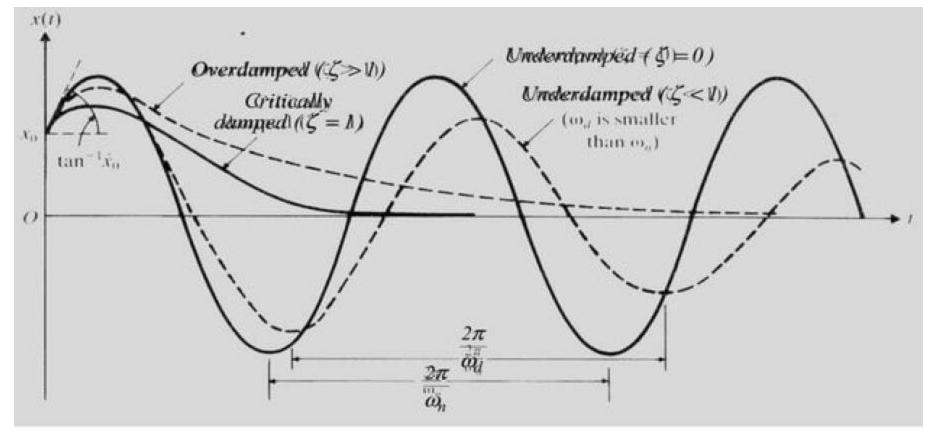
Critically damped systems have lowest required damping for aperiodic motion and mass returns to equilibrium position in shortest possible time.
